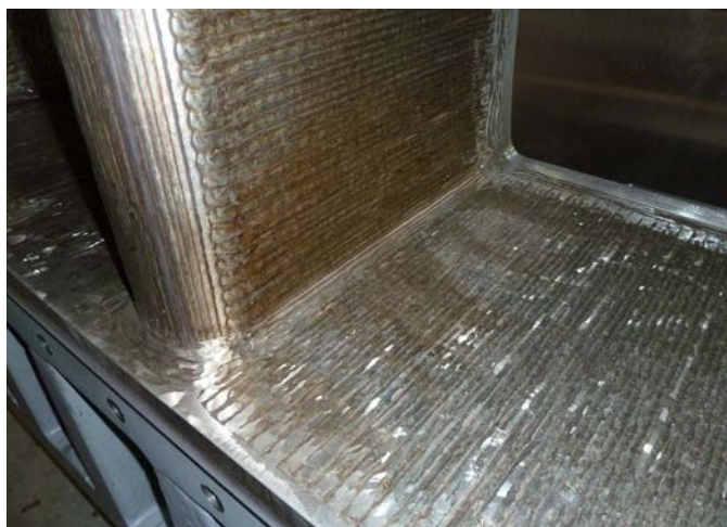
Cladding using Avesta FCW 309L-PW (E309T1-4/1) for high surface quality, also when welding out of position.
