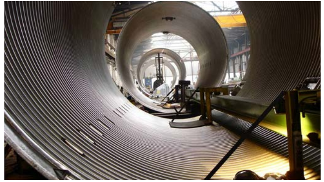
Welding of limpet coils with Ø 1.2 mm using BÖHLER EAS 4 M-MC (EC316L). Courtesy: Neuman Anlagentechnik, Germany
