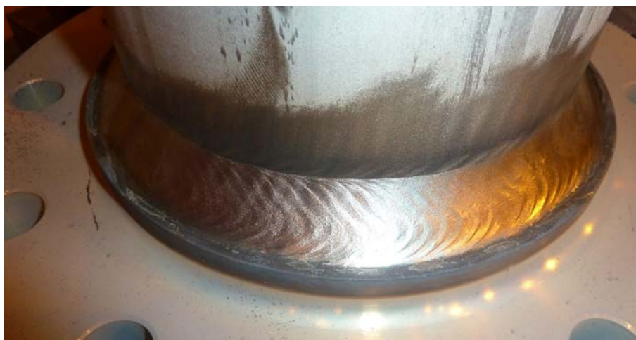
Fillet weld in flat position (PB / 2F). The base material is AISI 304L and the filler Avesta FCW-2D 308L/MVR (E308LT0-4/1). Ø 1.2 mm.
