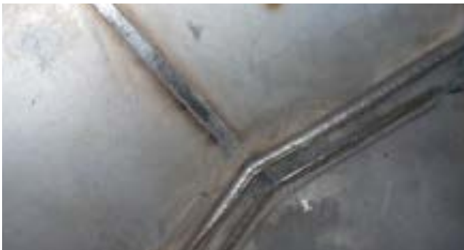
Welding of UNS S32205 in vertical-up and overhead position, using Avesta FCW 2205-PW (E2209T1-4/1).
