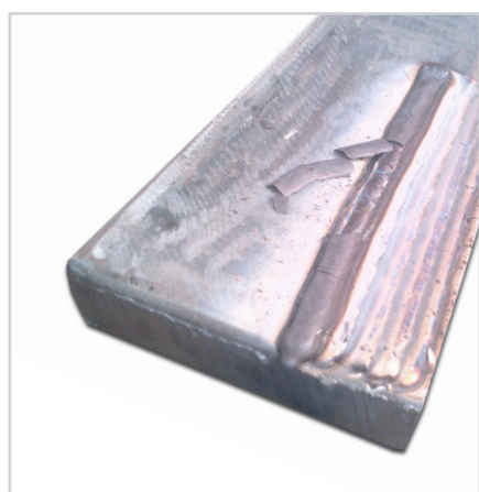
First layer cladding with BÖHLER E 309L H-FD (E309LT0-4/1) with good slag detachability.
