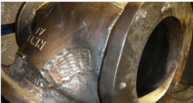
Avesta FCW 2507/P100-PW NOR (E2594T1-4/1) used for the repair welding of cast superduplex stainless steel.
