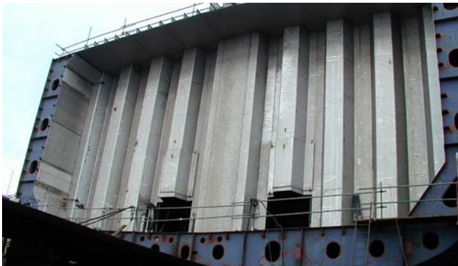
Cargo tanks in a chemical tanker made of UNS S32205 and welded using 100% CO 2 shielding gas. Welds in the flat and horizontal positions made with Avesta FCW-2D 2205 (E2209T0-4/1) using ceramic backing for the root pass. Avesta FCW 2205-PW (E2209T1-4/1) is used for welding out-of-position. Avesta FCW-2D 309L (E309T0-4/1) and Avesta FCW 309L-PW (E309T1-4/1) are applied for dissimilar welds.
