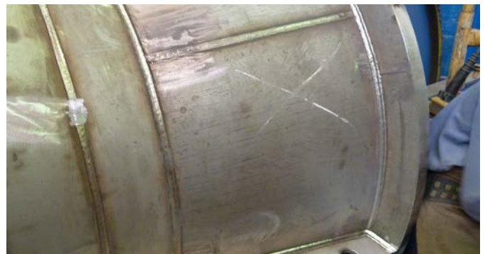
Seawater pump in UNS S32205 duplex stainless steel welded with Avesta FCW 2507/P100-PW (E2594T1-4/1) for highest possible corrosion resistance.
