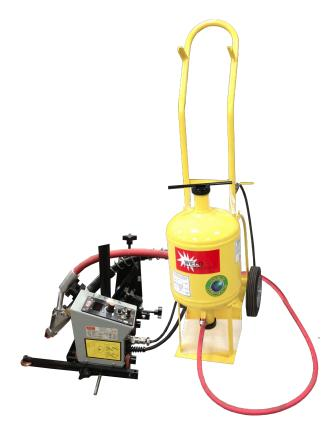
The MOGGY® for submerged arc welding is a continuous welding carriage suitable for use with portable pressure tank feed system. The minimum access requirement is 15" (381 mm) between vertical surfaces.
