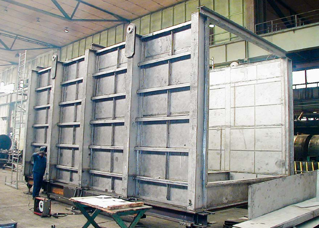
Stainless steel construction ready for pickling.
