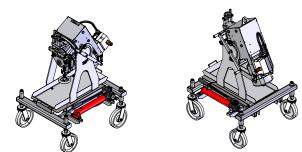
Bevel both top and bottom of the plate with one reversible bevelling machine. Lockable pivot system allows the beveller to work on the top or bottom side of the plate, reducing material handling providing increased productivity and cost savings in applications which require two sided bevelling.
